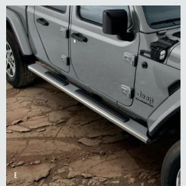
DOOR SILL GUARDS. Additional protection against scratches and scuffs. Feature an etched honeycomb background and Gladiator logo on the front door guards. Set of four.
